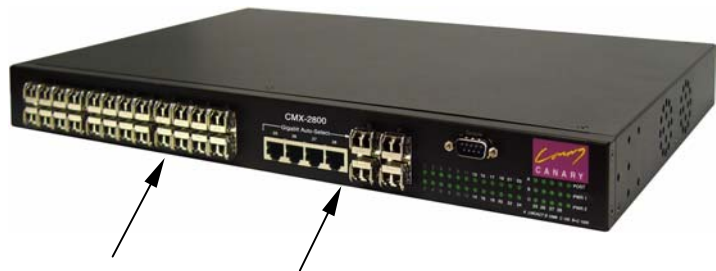
CMX-2800 Layer-3, Access Switch With 28 Ethernet Ports
