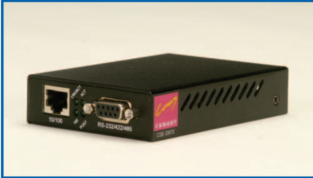
Illustrated: Serial 232 / 422 / 485 to Ethernet converter
